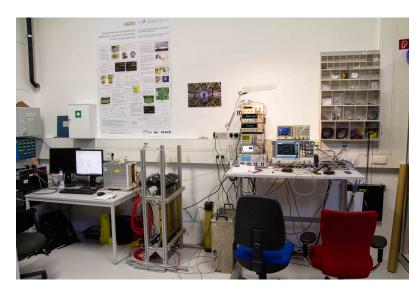
**Figure 4.1:** The new test set-up to characterize calorimeter type detectors and their readout electronics at GSI Helmholtzzentrum für Schwerionenforschung in Darmstadt. Left: computer terminals, remote high voltage supplies; Middle: Calorimeter modules and support structure; Right: low voltage supplies, pulse generators, oscilloscope, TRBv3 readout board.
