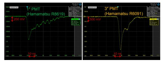
Figure 4.11: Raw pulse shapes for cosmic muons of ECAL modules equipped with a 1 inch HAMA-MATSU R8619 (left) and 3 inch HAMAMATSU R6091 PMT (right).
