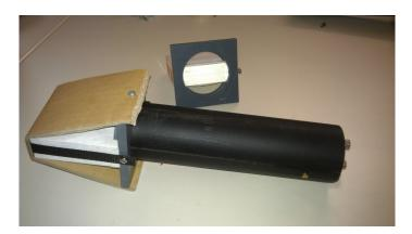
**Figure 4.4:** Photography of a scintillation trigger used to trigger cosmic muons. One can identify the plastic scintillator, warped in paper (Tyvek<sup>®</sup>), which is mounted to a PMT (HAMAMATSU H1949).
