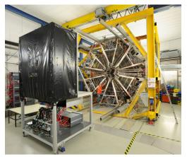
**(b)** Back-view: Pre-SHOWER detector (right) and Forward hodoscope Wall (left).
