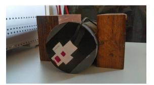
Figure 4.2: Top (left) and front (rigth) view of the PMT test-box, which allows to characterise 3 inch HAMAMATSU R6091 PMT with LED light.
