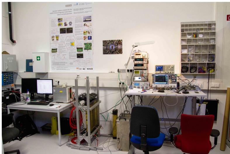
**Figure 4.1:** The new test set-up to characterize calorimeter type detectors and their readout electronics at GSI Helmholtzzentrum für Schwerionenforschung in Darmstadt. Left: computer terminals, remote high voltage supplies; Middle: Calorimeter modules and support structure; Right: low voltage supplies, pulse generators, oscilloscope, TRBv3 readout board.
