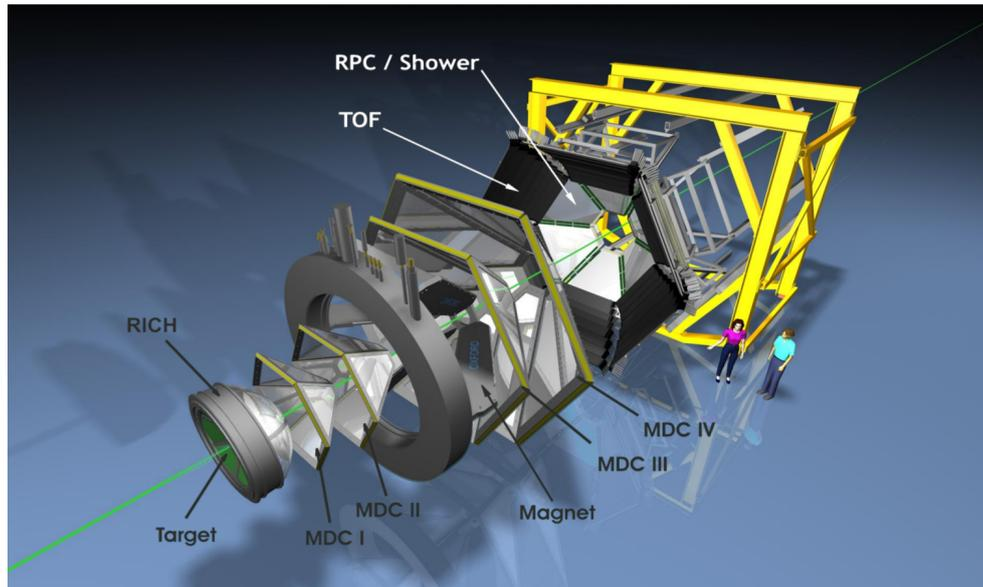
Figure 1.3: Expanded view of the HADES detector.
