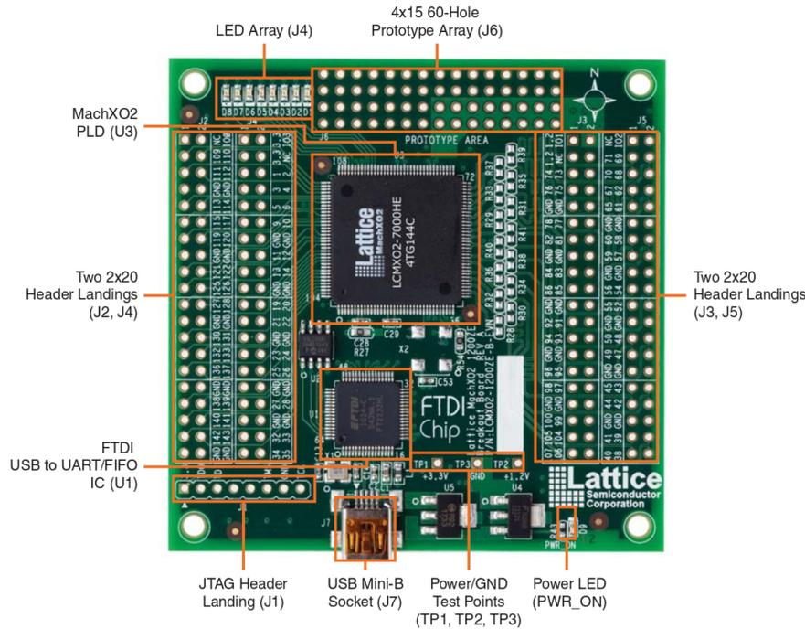
Figure 4.1: MachXO2 Breakout Board: top side [21].
