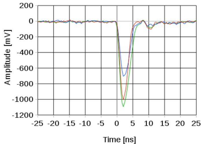
Figure 5.10: Signals from the HADES start diamond detector.
