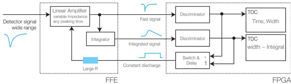
Figure 2.7: Sketch of the read-out system proposed for the ECAL. Signals after amplification are processed in the charge to width conversion system followed by the time digitization circuit which consists of two branches, one for fast timing and the second one for a pulse-width measurement which encodes the charge. Thus, two TDC channels are needed for one detector input channel.
