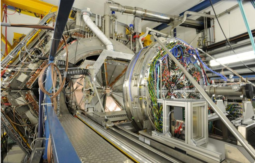
Figure 1.4: The HADES cave, front-view (in beam direction): the RICH detector (right) and the innermost MDC plane (left).
