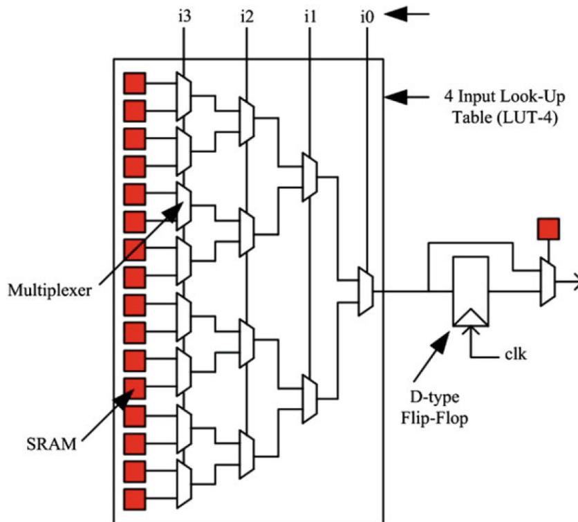
Figure 3.2: Basic logic element in an FPGA [20].
