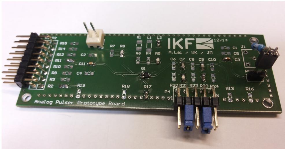
Figure 6.1: Prototype of the analog board for the hybrid pulse generator.
