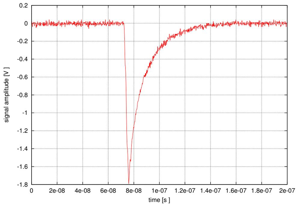
Figure 6.7: Output pulse produced by the real circuit when  $R = 0.39 \text{ k}\Omega$  and  $C = 189 \text{ pF}$ ; digital pulse width is set to 1.25 ns.
