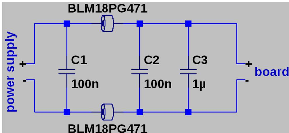
Figure 6.2: Filter for the power supply line.
