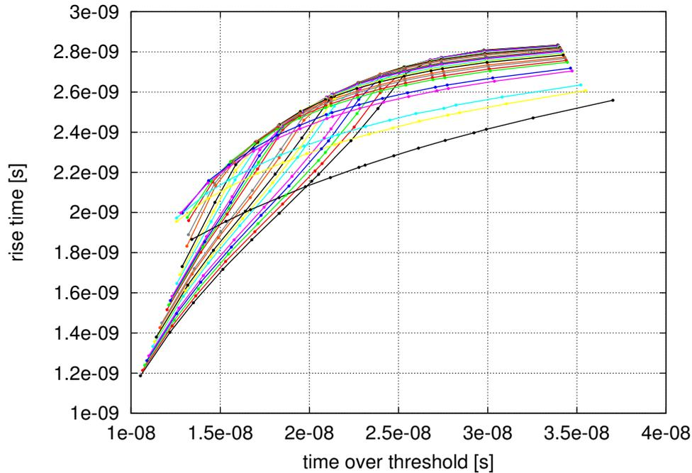
Figure 5.9: Rise time as a function of the time over threshold for all the possible combinations with the chosen discrete components.
