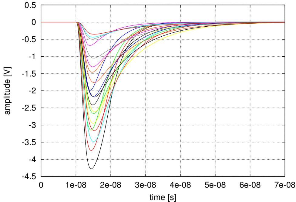
Figure 5.8: Simulation of the flexible analog circuit with  $R_{eq} = 0.39, 0.56, 0.82, 1.8, 6.8 \text{ k}\Omega$ ,  $C_{eq} = 68, 124, 150, 207 \text{ pF}$  and pulse width = 1.25 ns.
