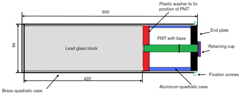
Figure 2.2: Schematic view of the calorimeter module.
