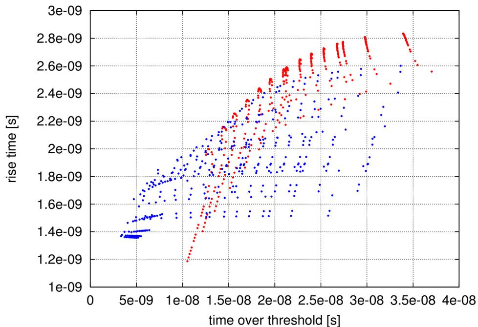
Figure 5.13: Rise time as a function of the time over threshold for all the possible combinations with the chosen discrete components: red dots correspond to the asymmetric pulses and blue dots correspond to the more symmetric pulses.
