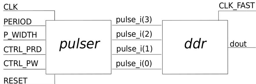
Figure 4.4: Function block diagram for the fast version of the pulse generator.
