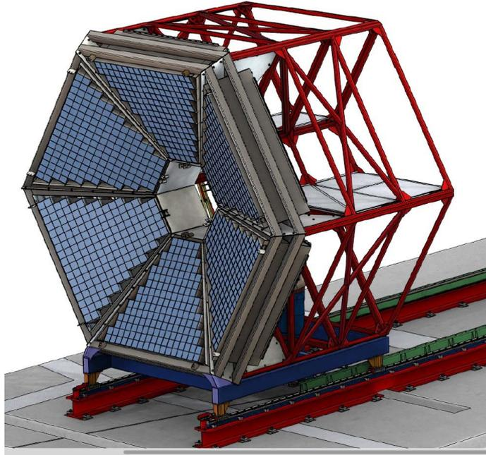
Figure 2.4: 3D model of the ECAL mounted on its support structure.
