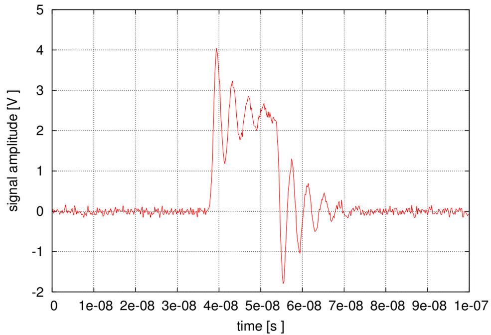
Figure 6.5: Input signal to the analog board; digital pulse width is set to 25 ns.
