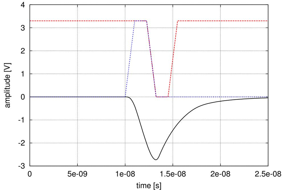
Figure 5.11: Digital input pulses with opposite polarity, one delayed with respect to the other; output pulse shows a shorter tail (red).
