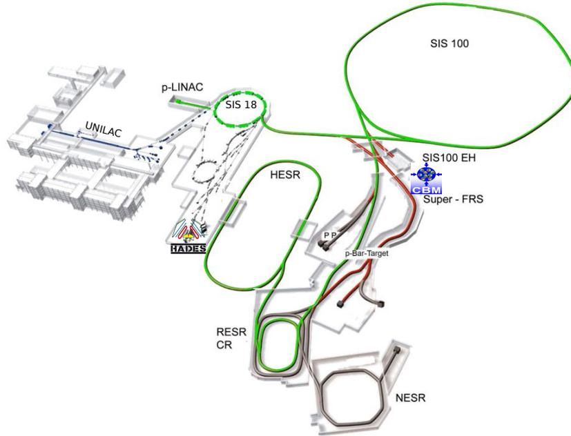
Figure 1.2: The existing GSI facility (grey) and the planned future facility FAIR (green and red) [6].
