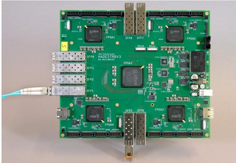
Figure 2.6: The Trigger and Read-out Board version 3.
