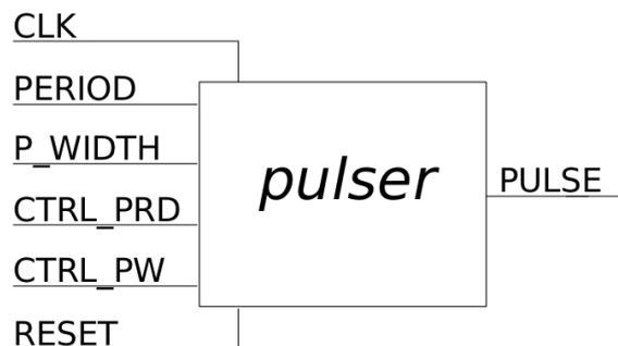
Figure 4.2: Function block diagram for the basic pulse generator.
