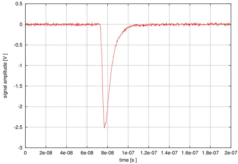
Figure 6.6: Output pulse produced by the real circuit when  $R = 0.39 \text{ k}\Omega$  and  $C = 39 \text{ pF}$ ; digital pulse width is set to 1.25 ns.
