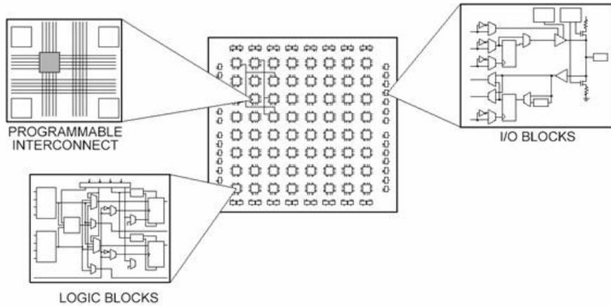
Figure 3.1: Basic scheme of an FPGA.
