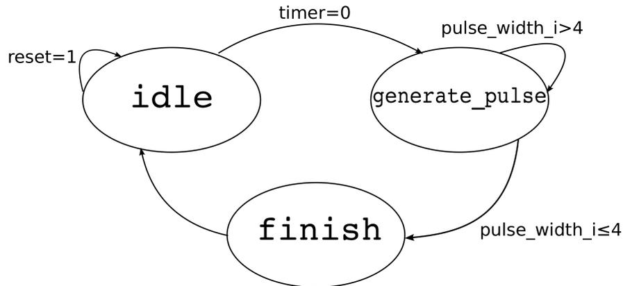
Figure 4.5: Diagram of the Finite State Machine used to implement the architecture of the *pulser*.
