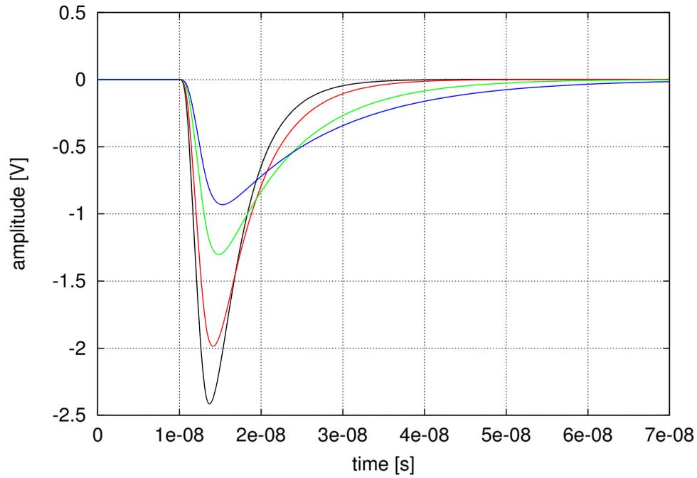
Figure 5.5: Simulation of the analog circuit with  $R1 = 1.8 \text{ k}\Omega$ ,  $C3 = 39$  (black), 68 (red), 150 (green), 245 pF (blue) and pulse width = 1.25 ns.
