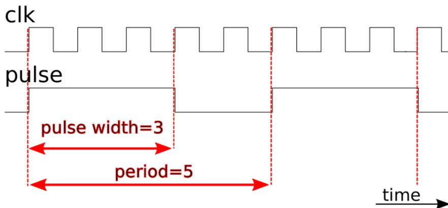
Figure 4.3: Signal representation of the clock signal and the pulse generated synchronously with its rising edge.
