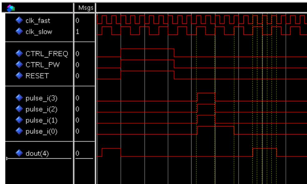
Figure 4.7: Simulation of the fast pulse generator: pulse width is set to five.
