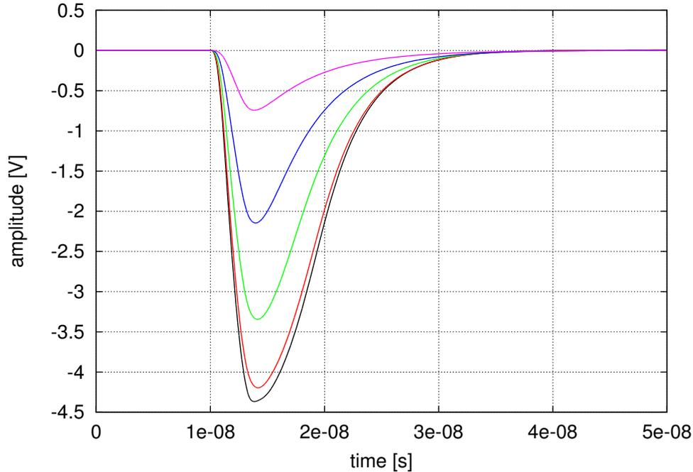
Figure 5.4: Simulation of the analog circuit with  $R1 = 0.39$  (black),  $0.47$  (red),  $0.82$  (green),  $1.8$  (blue),  $6.8 \text{ k}\Omega$  (violet),  $C3 = 56 \text{ pF}$  and pulse width =  $1.25 \text{ ns}$ .
