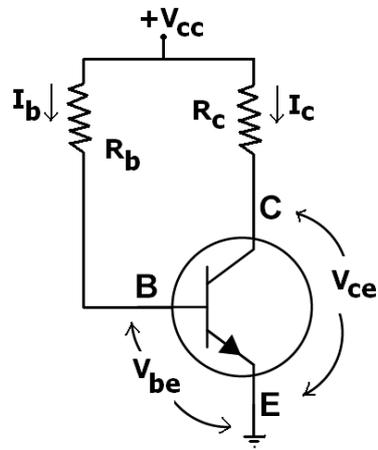
Figure 5.2: Bipolar transistor with fixed bias [29].
