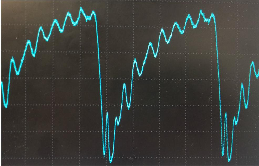
Figure 6.3: Screenshot from the oscilloscope shows the amplitude versus time of the hybrid pulser output signal (arbitrary units).
