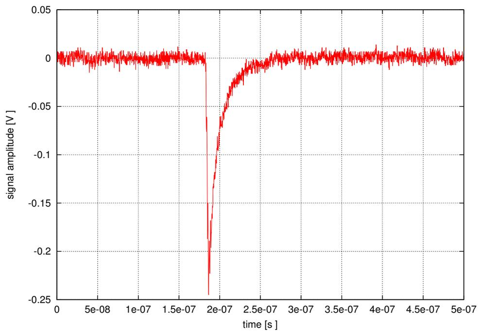
Figure 6.8: Output pulse produced by the real circuit when  $R = 6.8 \text{ k}\Omega$  and  $C = 39 \text{ pF}$ ; digital pulse width is set to 1.25 ns.
