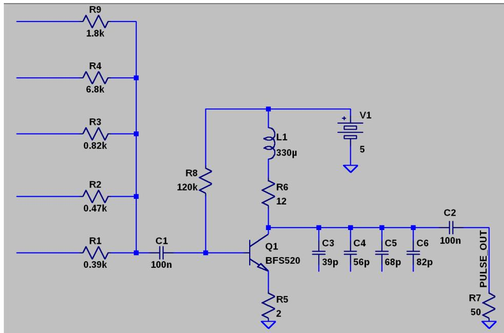
Figure 5.7: Schematic of a more flexible analog circuit to be connected to the outputs of the FPGA to perform testing of the PADIWA AMPS board.
