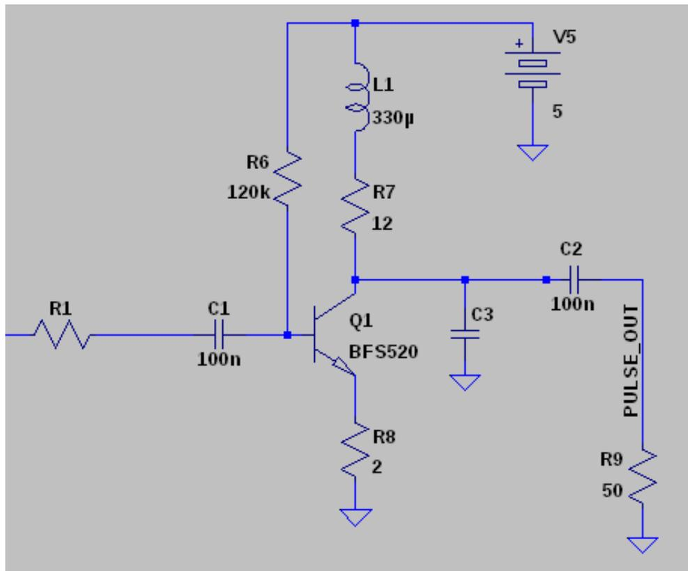
Figure 5.3: Schematic of the analog circuit to be connected to the outputs of the FPGA to perform testing of the PADIWA AMPS board.
