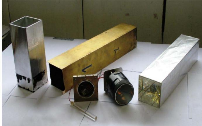
Figure 2.3: A disassembled ECAL module: the brass housing (left), the lead glass block (right), the high voltage divider and the PMT (middle).
