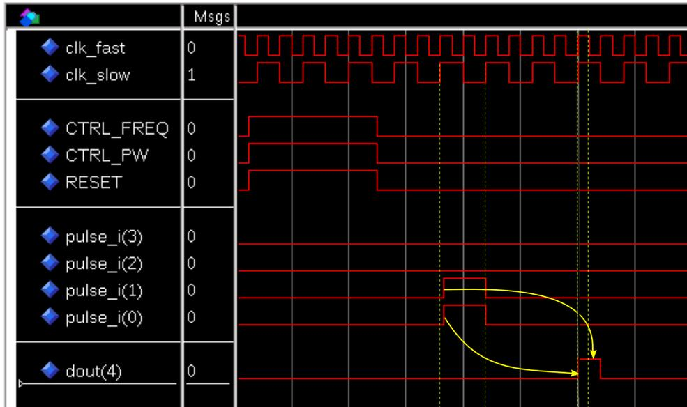
Figure 4.6: Simulation of the fast pulse generator: pulse width is set to two.
