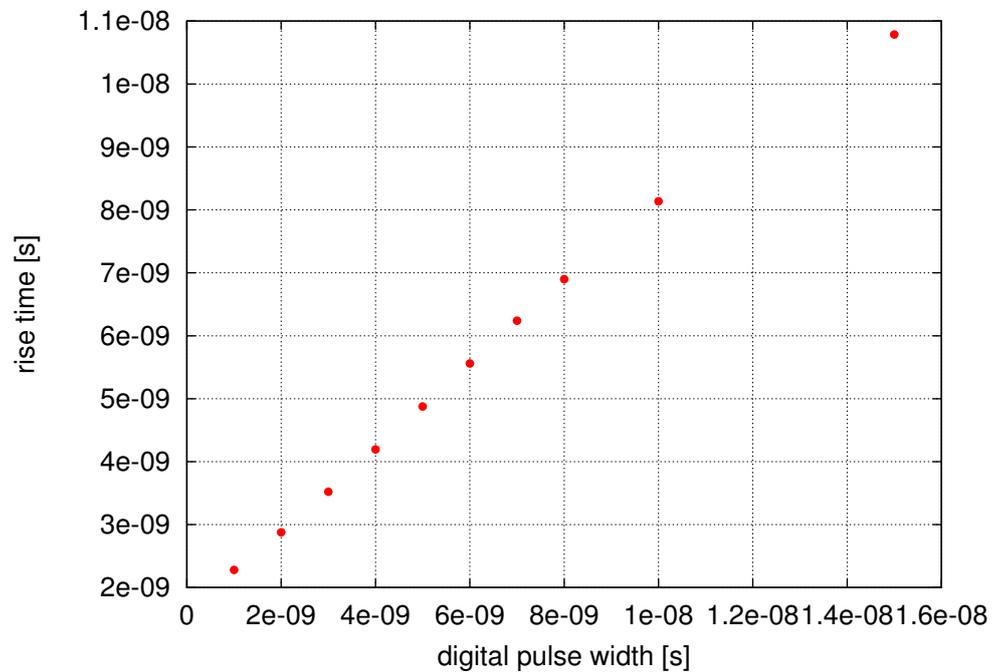
Figure 5.6: Rise time as a function of the digital pulse width for  $R1 = 1.8 \text{ k}\Omega$  and  $C3 = 150 \text{ pF}$ .
