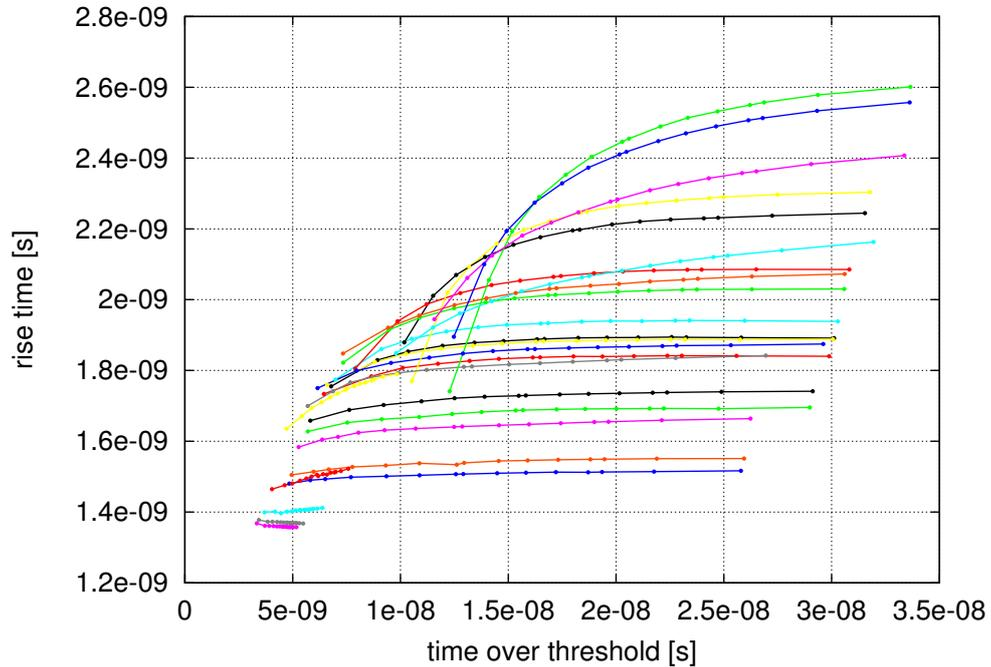
Figure 5.12: Rise time as a function of the time over threshold for all the possible combinations with the chosen discrete components for more symmetric pulses.
