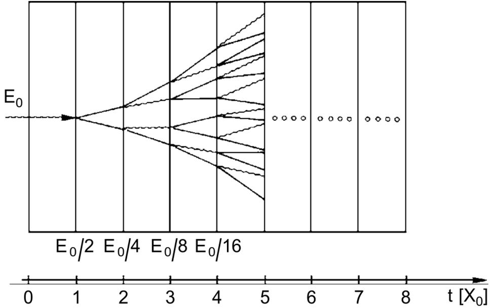
Figure 2.1: Sketch of a simple model for shower parametrisation: the wavy lines are photons and the solid lines electrons or positrons [10].
