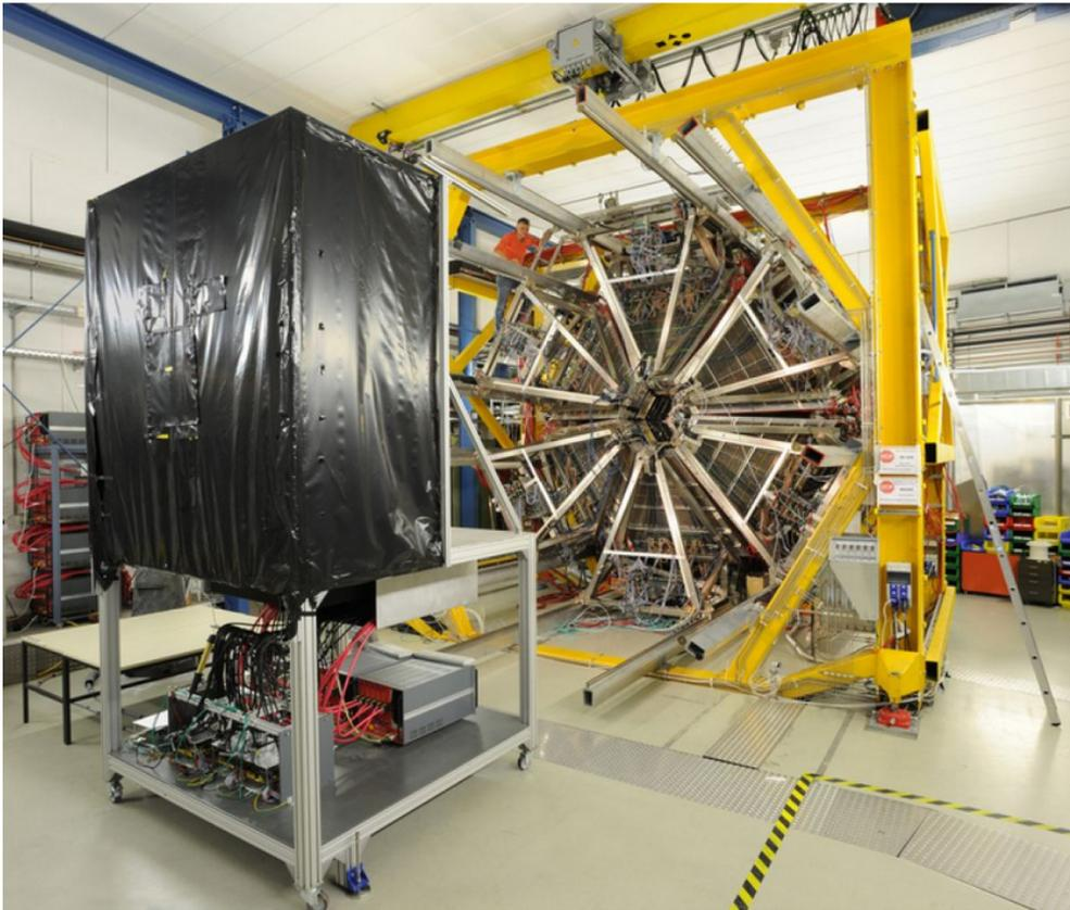
Figure 1.5: The HADES cave, back-view (in beam direction): Pre-Shower detector (right) and Forward Wall (left).
